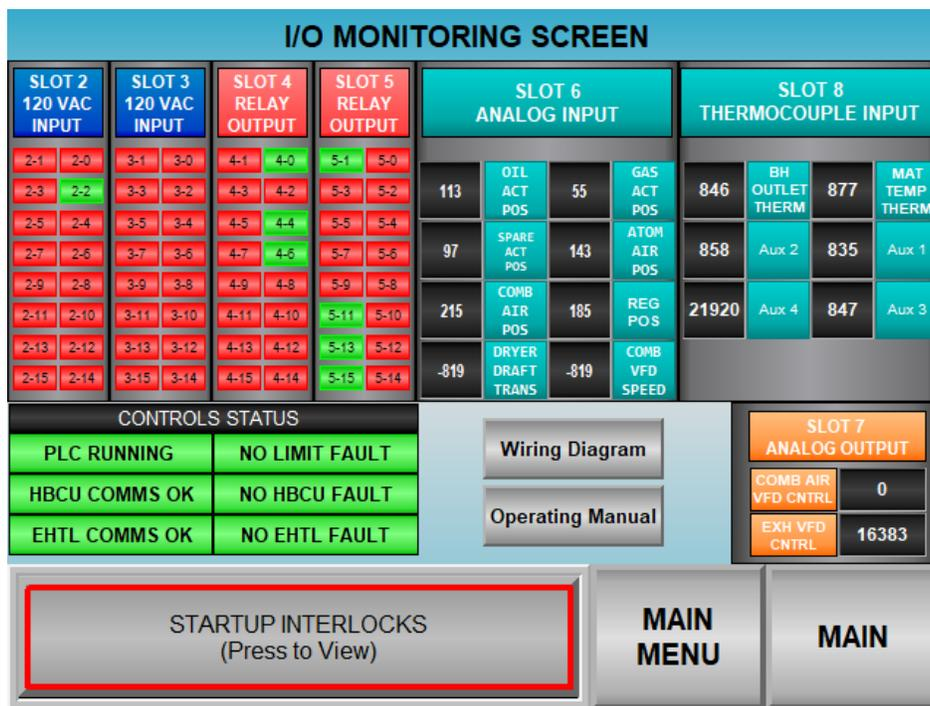
The I/O Status screen can be accessed by pressing the **I/O REF SCREEN** button that is within the **MAIN MENU**. From this screen you can monitor the status of all of the input and output modules, as well as monitor the communications status between the PLC, the Honeywell Burner Control Unit (HBCU) and the Exhaust High Temperature Limit (EHTL).
