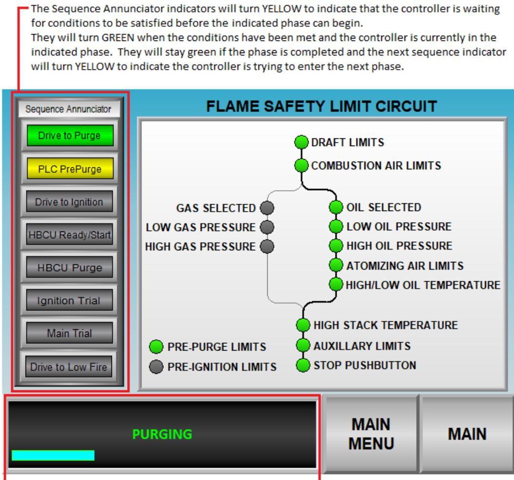
The local message display will indicate which limit has opened and will also indicate the phase it is in, in all screens.
