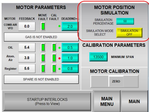
**\*\*\*If the Combustion Air VFD is enabled it must be running to operate in Simulation Mode.\*\*\***
