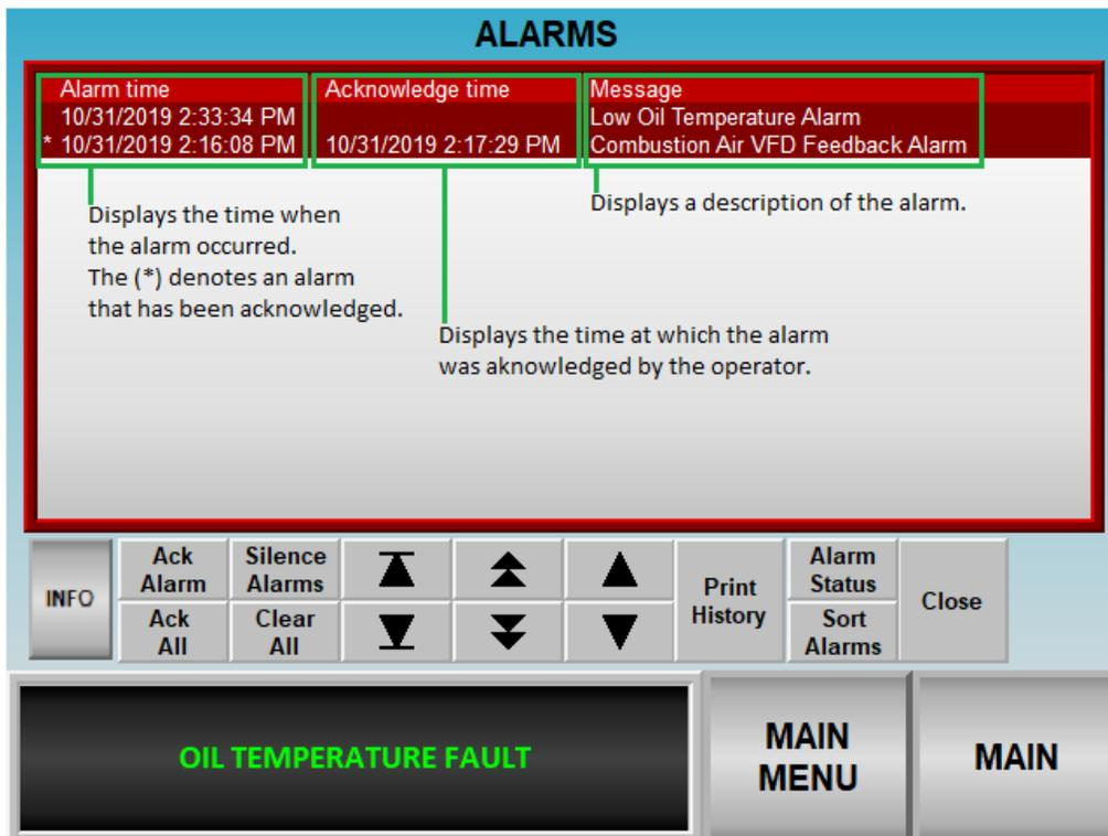
**INFO:** Pressing this button will open a pop-up window that will display a Diagnostics Log that is generated by the HMI, the messages here relate to display operating system or communication errors.
