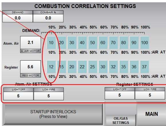
Since the Combustion Air element is the controlling lead (*damper or VFD*) its position will be at 10% of the calibrated span (*due to the Simulation Demand Percentage being set at 10%*).
