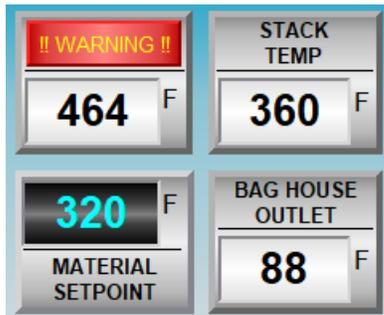
These warning beacons are only a visual warning indicating that the temperatures are approaching critical levels, if these temperatures continue to increase, the burner will automatically drive to Low Fire, trip the High Limit device or could cause critical damage to the Baghouse filters.
