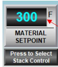
Pressing the setpoint panel digits (blue) will open a numerical entry panel, from here you can adjust the setpoint of the current temperature mode (*setpoints can also be adjusted in the Controller Setup menu*).
