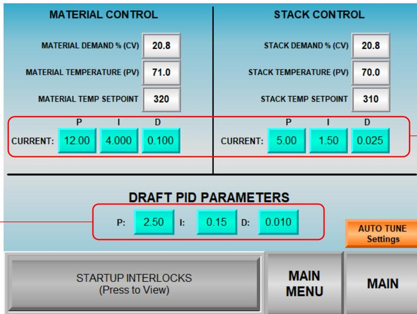
To observe how changes made to the Draft PID Parameters are affecting the Draft Control you will need to switch to the Main Screen and watch the Draft VFD Speed relative to the Draft Pressure readings from there.
