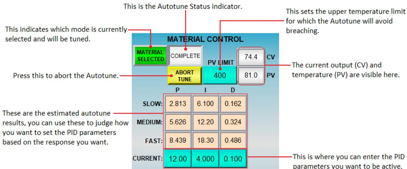
**Material/Stack Mode Selection:** You can press these buttons to select between the Material or Stack temperature Autotune Mode. In the above example the Material Mode is selected, pressing this button in the Stack Control panel will switch to Stack Control mode and the indicator will change to green in the Stack Control panel.
