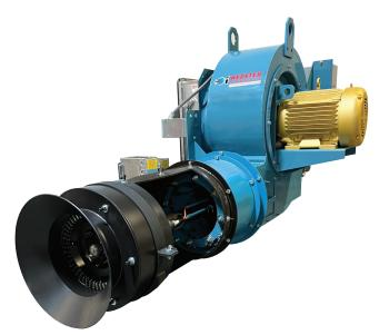
The Webster Combustion Twister series is an open-fired register-style burner that allows the user to shape the flame by controlling the register vanes to optimally fit their dryer and combustion zone. This flame shaping capability means the flame will not impinge on the material, and CO can be maintained at lower levels. The Twister register can be controlled using either a servo or linkage to shape the flame quickly and easily during start-up, or when mix changes may require a change in setup.
